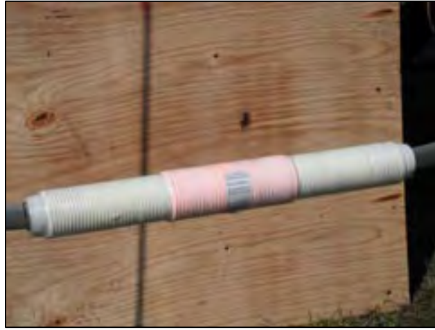
An example of an Implosive Splicing device used to weld powerline sections together. Photograph courtesy of Eversource
